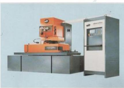
Figure 5. Wire cutting machine
