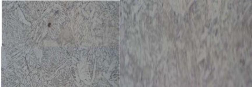
Figure 21. Microstructures in HAZ (b)
