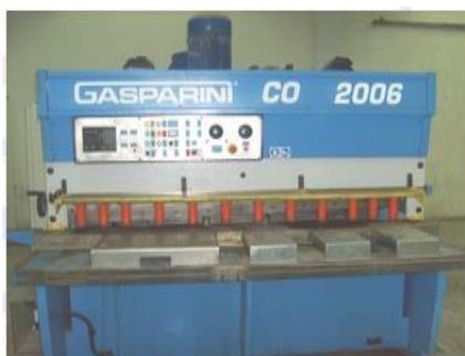
Figure 4. Shear cutting machine
