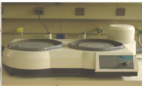
Figure 7. Grinding machine
