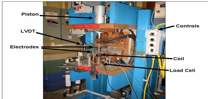
Figure 1. Centerline AC RSW apparatus
