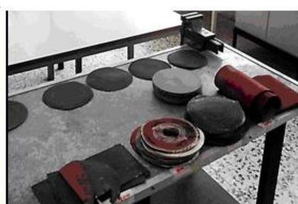
Figures 8(a). Polishing machine (b) Grinding and polishing disc
